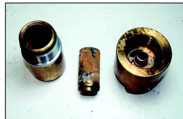
CFC 50 Series Brass Tee Filter after modified ASTM G-175 testing at 5000 psig oxygen.
