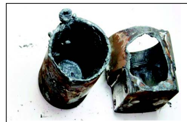
316 SST Tee Filter after modified ASTM G-175 testing at 3000 psig oxygen.
