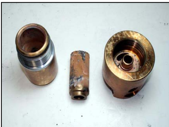
CFC 50 Series Brass Tee Filter after modified ASTM G-175 testing at 5000 psig oxygen.
