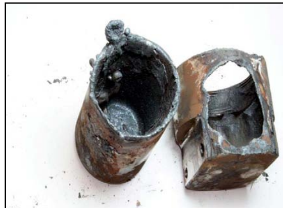
316 SST Tee Filter after modified ASTM G-175 testing at 3000 psig oxygen.
